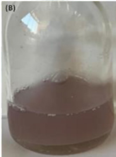
Fig. 3. The biogenic synthesized ZrNPs. The light violet color was changed to dark purple after 24h incubation [flask (A) is the control (cell-free filtrate without zirconia cations), and flask (B) is the test flask (cell-free filtrate with zirconia cations ZrF6)]
